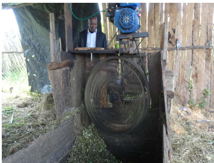
Figure 5 A demonstration of a biogas powered chaff-cutter being used to cut Napier grass from the SGP supported biogas projects in Kieni, Nyeri County
