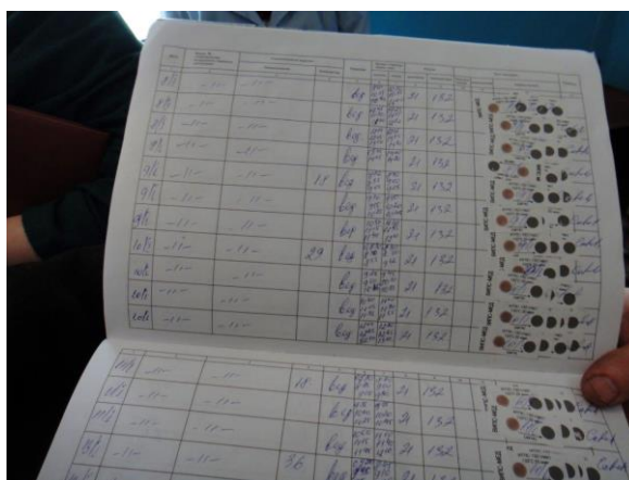
Photo 4: Records are kept for each batch autoclaved and the indicators on the right verify that the sterilisation was successful.
