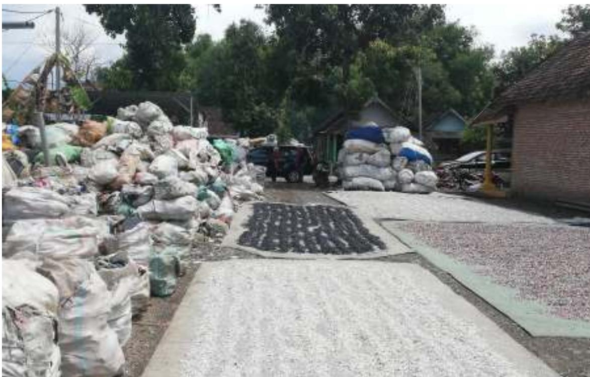
Figure 1. In the Kajagan village, Mojokerto, several farmers shifted from agriculture to plastic recycling. Here, shredded plastic after floating selection drying at the sunlight.
