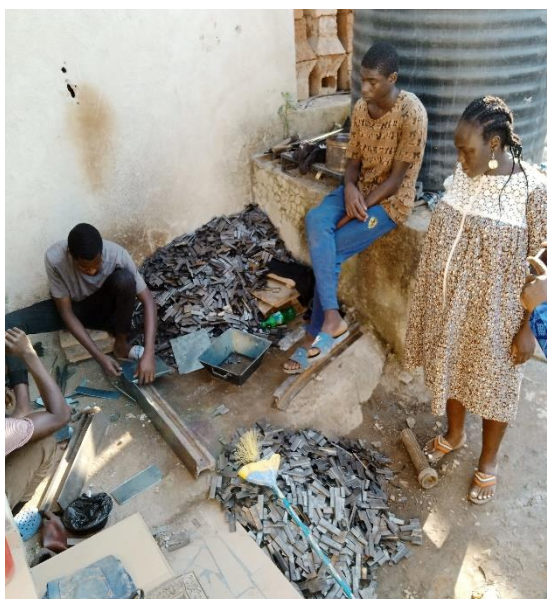
Photo 10 - Rails for cutting and bending of cookstove parts
