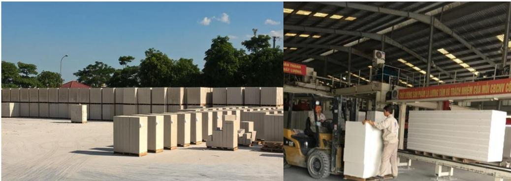
**AAC bricks and AAC panel produced at Viglacera**
