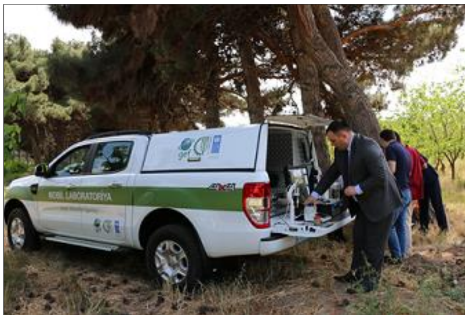
Figure 8: Photograph of mobile laboratory in use, analyzing soil samples at cereal field 11
