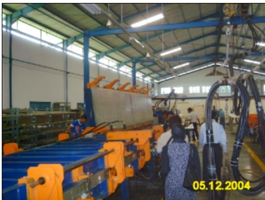
Photo 1: Manufacturing line, PT Far East (Indonesia) Refrigeration plant, Jakarta. The company produces 12,000 m 3 of polyurethane sandwich board per year. They received several high pressure foam dispensers under the UNDP project Sector Phase-out Plan for Elimination of CFCs in the Refrigeration (Manufacturing) Sector , and their products are now CFC-free.
