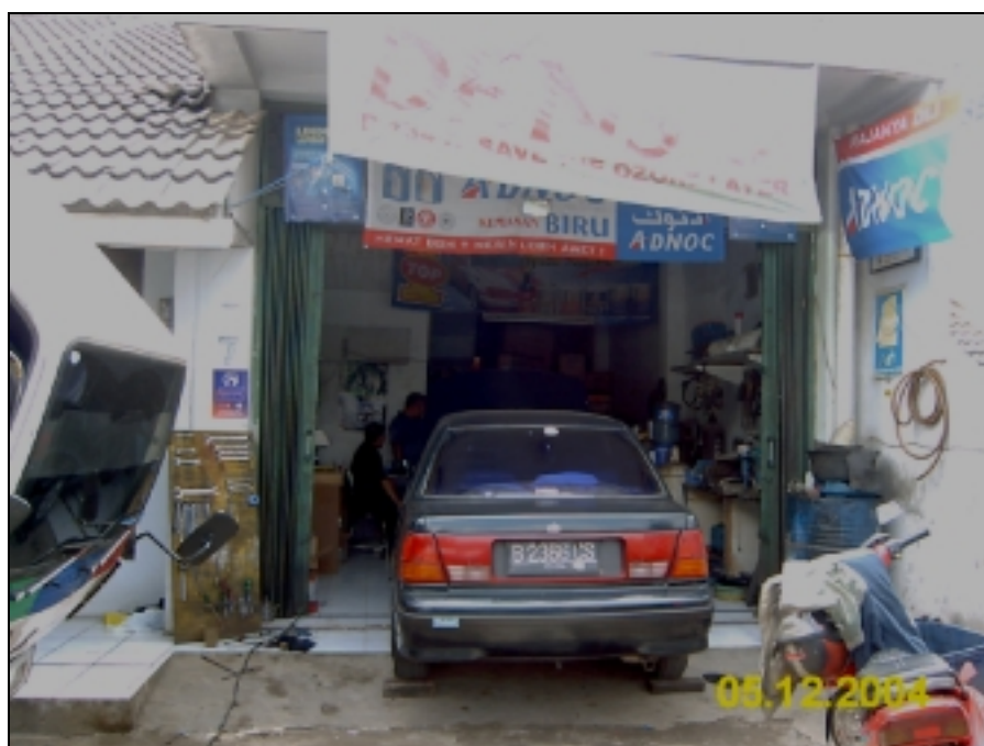
Photo 4: Tjahja Motors, Jakarta. This small facility injects polyurethane foam into refrigeration trucks, boats and facilities at the customer's sites. UNDP provided a portable CFC-free polyurethane foam injector.
