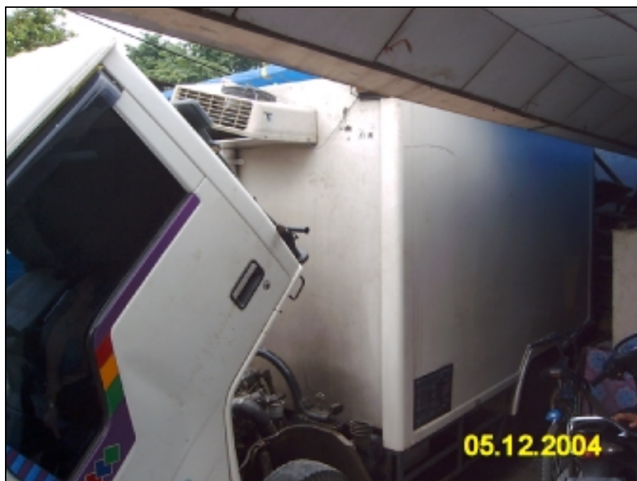
Photo 5: Refrigerator truck belonging to Tjahja Motors. The insulation in this vehicle was injected on site, a typical process undertaken by the company.
