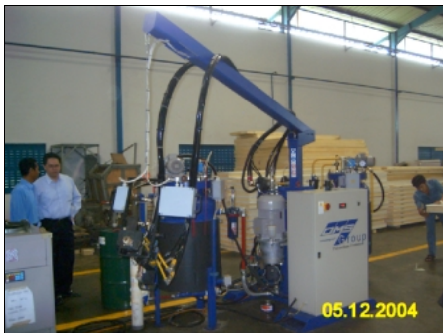
Photo 2: High pressure polyurethane injector provided to PT Far East (Indonesia) Refrigeration by UNDP. The company is interested in participating in a CFC-free promotional campaign that would educate their customers on the advantages of purchasing from certified CFC-free producers.
