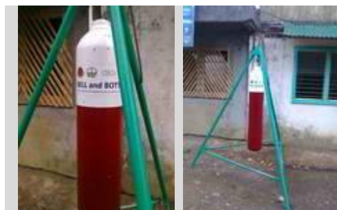
Bell and Bottle, a low-cost Early Warning System installed in Barangay Nogotgot, Manito, Albay.
