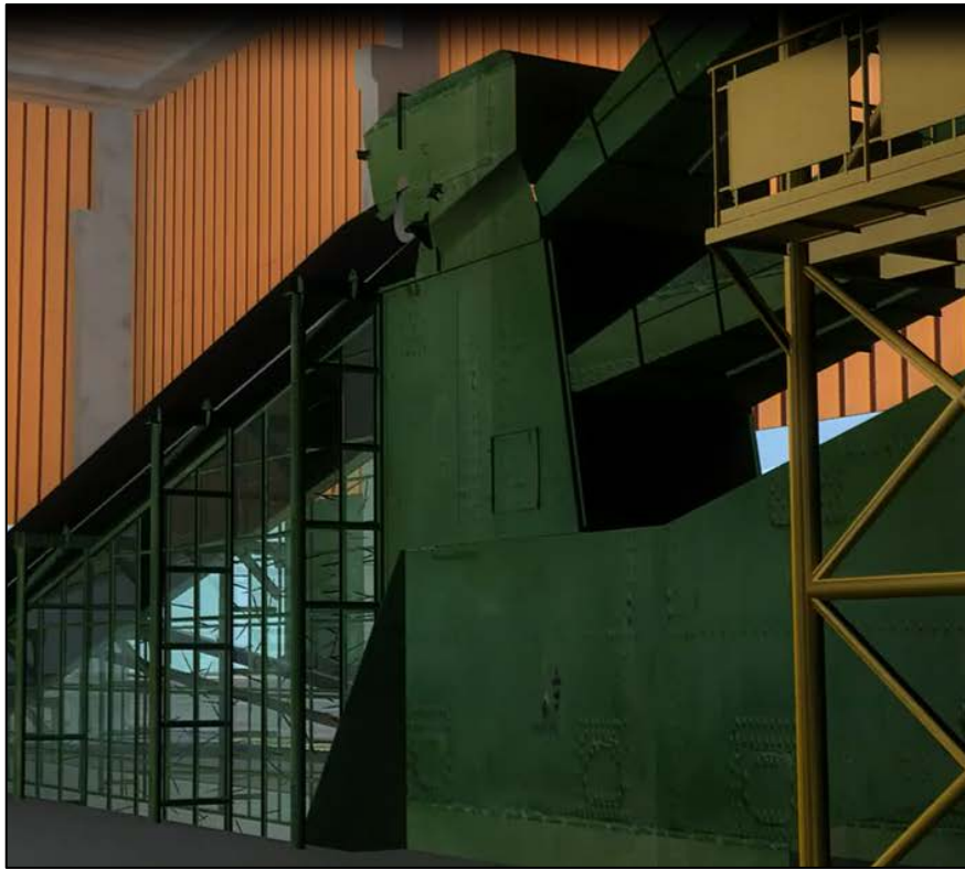
Figure 2. Chopped cane trash separator, Usina Alta Mogiana (CAD photo, from Hassuani, 2013)
