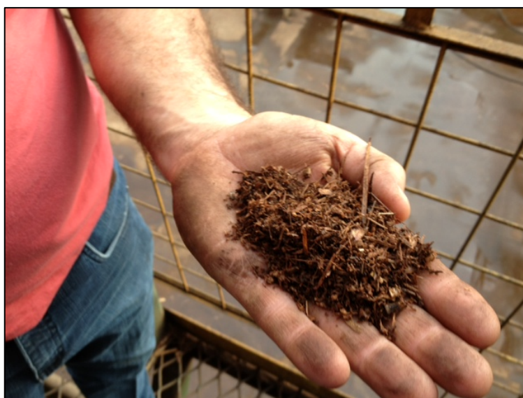
Figure 4. Mineral and organic impurities separated in dry cleaning system, Usina Alta Mogiana, 2013
