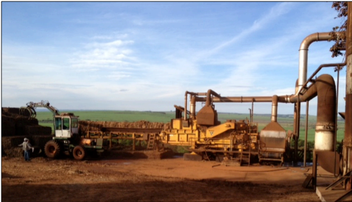
Figure 8. Bales dismantling and trash shredding system, Usina da Pedra, 2013
