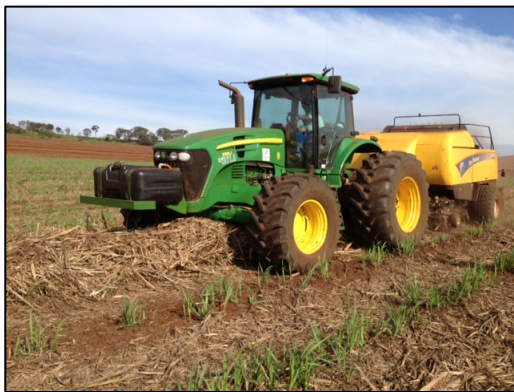
Figure 6. Baler collecting trash and downloading a bale, Usina da Pedra, 2013
