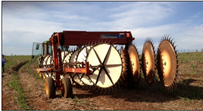
Figure 5. Mechanical rake utilized for preparing rows of trash, Usina da Pedra, 2013
