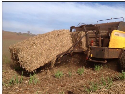
Figure 6. Baler collecting trash and downloading a bale, Usina da Pedra, 2013
