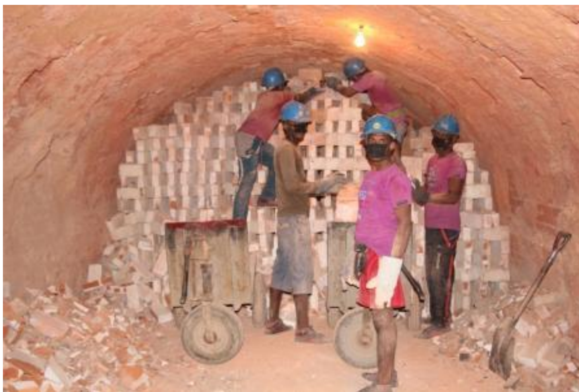
Exhibit 3-1: Universal, PDF-B Demo Hybrid Hoffman Kiln (HHK) – kiln unloading; visit gave impression of well-run operation and employees satisfied with the opportunity. (MTR mission, Oct. 2014, photo by Shamim Iftkhar)
