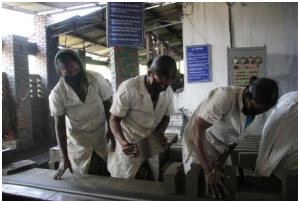
Exhibit 3-2: Universal - PDF-B Demo Hybrid Hoffman Kiln (HHK) – brick formation line (MTR mission, Oct. 2014, photo by Mr. Shamim Iftakhar, IKEBMI Communications Officer)
