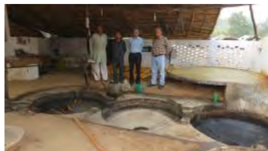
Energy efficient 3 pan Jaggery furnace
