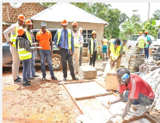
Transforming stone dust into tiles at Kyogo Mazinga (StoneCraft) Ltd
