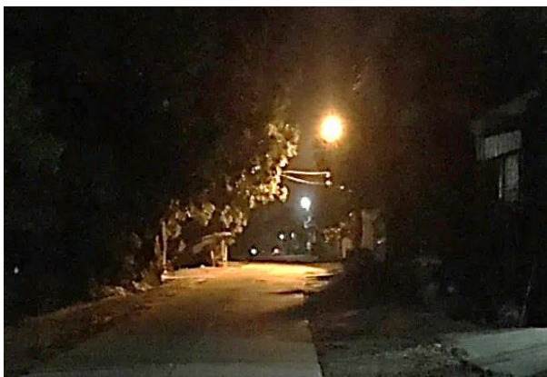
Street light system in the Thai Nguyen city before and after replacing HPS lamp with LED lamps produced by Rang Dong Light Source and Vacuum Flask JSC (replaced 150W HPS with 120W LED lamps). Total power of HPS lamps: 9.450 kW, total power of LED lamps: 5.040 kW; The amount of electricity saved per year: 17.464 kWh.
