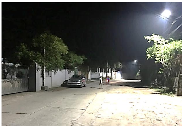
Street light system in the Thai Nguyen city before and after replacing HPS lamp with LED lamps produced by Rang Dong Light Source and Vacuum Flask JSC (replaced 150W HPS with 120W LED lamps). Total power of HPS lamps: 9.450 kW, total power of LED lamps: 5.040 kW; The amount of electricity saved per year: 17.464 kWh.
