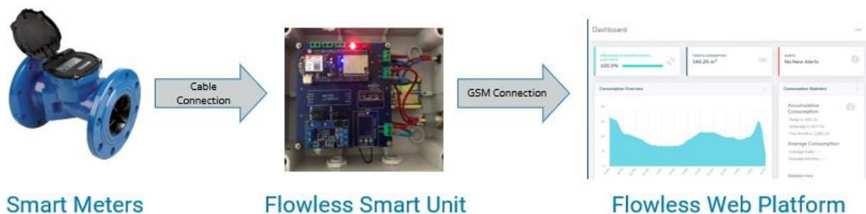
Figure 1. Flowless Smart System Structure
