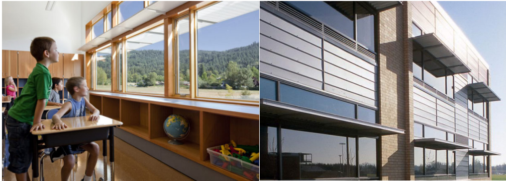
Figure 2.1. Intermediate light shelves reducing glare and evenly distributing daylight in a space 5
