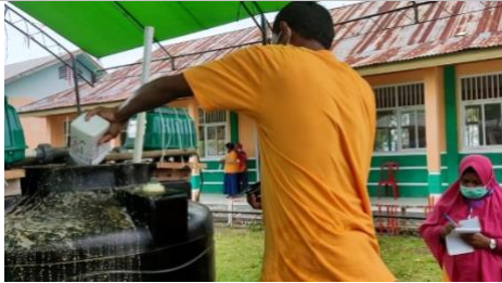
Figure 31. Addition of SMBS to reduce free cyanide
